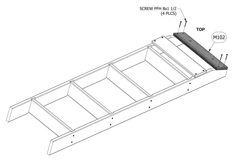
(1) M72 - ROCK WALL SLAT - W100023 5/8"x3 3/8"x20 1/4" (16x86x514) (2) H73 - ROCK WALL RAIL - W100024 1"x3 3/8"x48 3/4" (24x86x1238)
